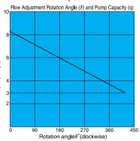
The values indicated above are at maximum pump discharge volume with the flow volume adjusting screw at the 0° position.
